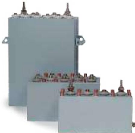
Medium & high frequency water-cooled / air-cooled capacitors are specially designed for use in inductive heating & melting plants for power factor improvement as also for tuning of the circuits for varying inductive loads. These capacitors are manufactured against order to meet the specific and exacting requirements of each customer. For the given application, the performance of these capacitors, demand extreme levels of Reliability, Safety and Life expectancy.
